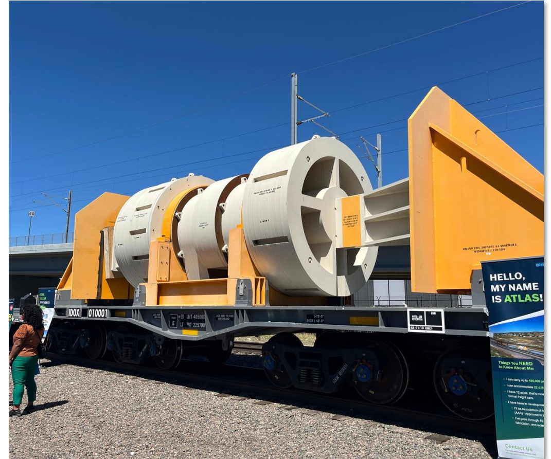
The Atlas rail car loaded with a test weight resembling a cask
