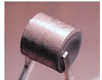
Typical fuel pellet loaded into a fuel rod (Tulenko).
