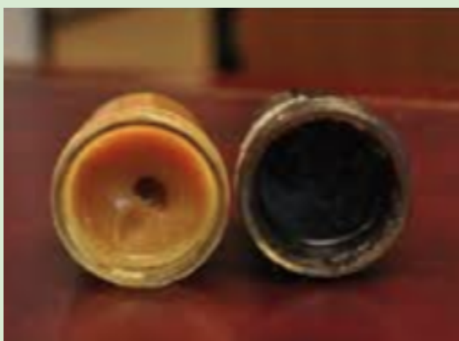
Waxy Crude Oil After Hardening
