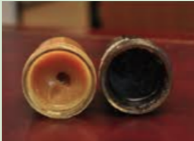
Waxy Crude Oil After Hardening
