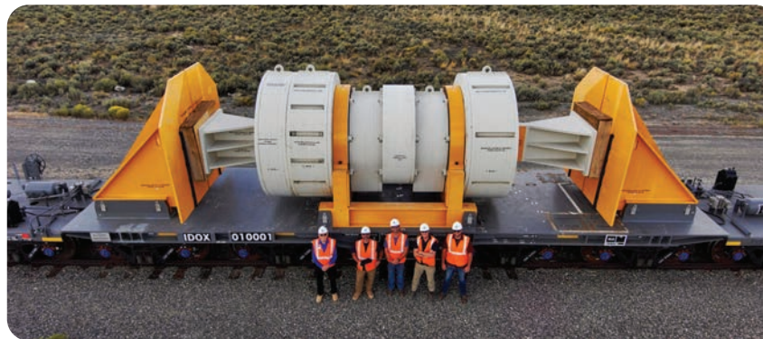
▲ Aerial shot of the Atlas rail-car carrying a test load simulating a shipment of used nuclear fuel
