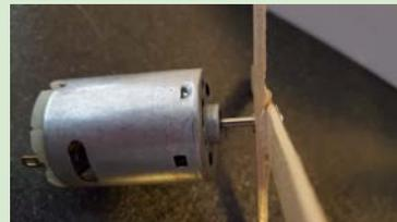
To help the students create the windmill portion, glue two craft sticks together in the middle. Once the glue has set, drill a hole in the middle so it will fit tightly around the drive shaft on the mini motor. You may want to have a drill during the building of the project in case students need to make some changes. It is also suggested to make extra cross pieces. You will also need to divide the students into groups of 3-4 students.
