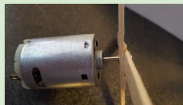
To prep the windmill portion, glue two craft sticks together in the middle. Once the glue sets, drill a hole in the middle. It should fit tightly around the drive shaft on the mini motor. A drill could be useful during the project in case students need to make some changes. It is also suggested to make extra cross pieces. You will need to divide the students into groups of 3-4 students.
