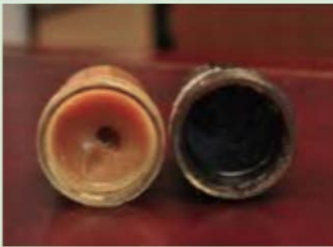
Waxy Crude Oil After Hardening
