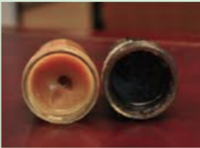
Waxy Crude Oil After Hardening
